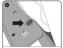
Lightly re-tighten the side panel mounting screw which as removed in Step 3. Recommended tightening torque: 1.1
