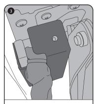
Align the screw holes of the footrest connection cover with those on the main unit.
