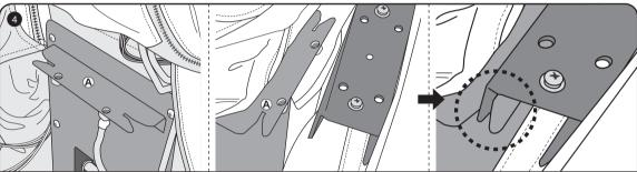
Attach the combined left side panels 6, 7, and 8 to the left side panel mounting receiver bracket (A) by hooking them onto the mounting hook bracket.
