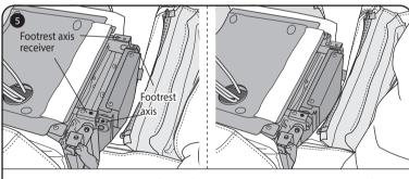
With the thread holes of the footrest axis facing upward, lift the footrest and set the footrest axis receivers of the main unit.
