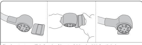
Place the caster stoppers, lift the front pipe of the caster slightly and push it in from the back.
