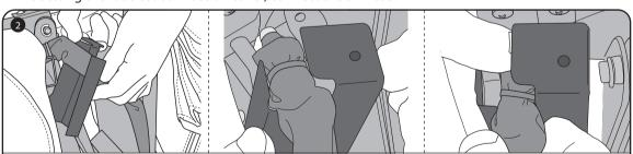
Pass the air hose through the notch (top) of the footrest connection cover from below. Hook the notch (bottom) of the footrest connection cover onto (B) on the main unit side, and push the tip of the air hose into the connection port by using your left index finger. Ensure the air hose is fully inserted.
