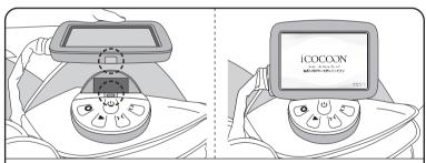
Remove the monitor and attach it to the main unit remote control (it attaches with magnets).
