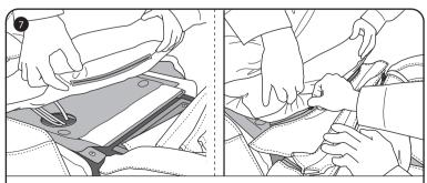
Lift the seat. Align the zipper at the upper end of the footrest cover with the main unit, and close the zipper.
