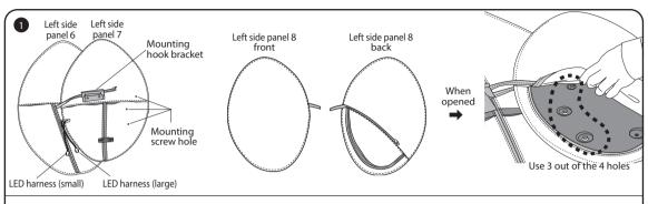
Turn the left side panel 8 to the backside, open the zipper, and attach left side panel 8 to left side panel 6 and 7.
