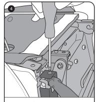
Use a Phillips screwdriver to tighten the screws on the footrest connection cover.
