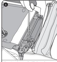
By using the supplied T-shaped wrench, securely fasten the footrest with the footrest mounting screws.
