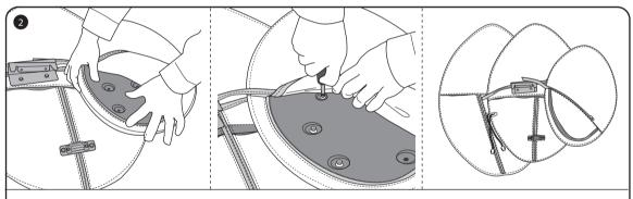
Align the holes (three places) in left side panel 7 with the holes (three places) in left side panel 8, and use your Phillips screwdriver to secure the side panel mounting screws. After securing, close the zipper on left side panel 8.
