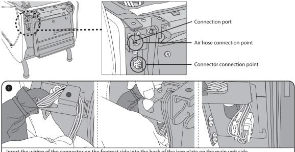
Insert the wiring of the connector on the footrest side into the back of the iron plate on the main unit side, and push it in until clicks into the place.
