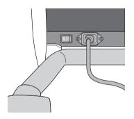
②Turn "ON" the main power switch located at the rear of the main unit. At this point, characters are displayed on the monitor, and the logo LED on the top panel will light up.
